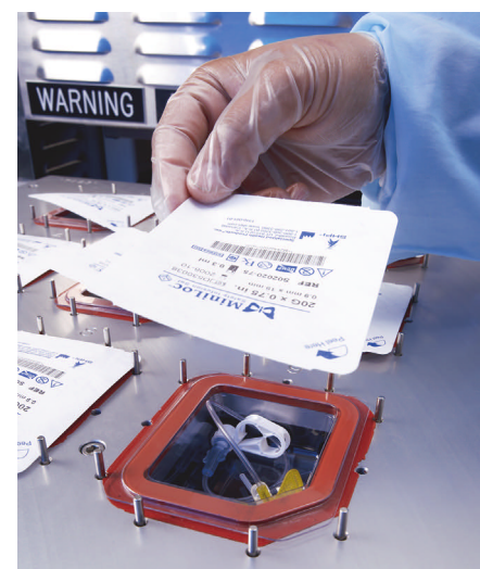
The geometry holding the product's wings changes angles along the vertical wall of the part. The vinyl compensates for changes.
