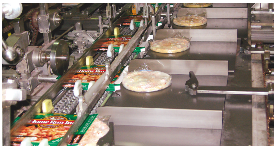
Above, the film-wrapped pizzas index into the cartoner, where pusher arms insert them into cartons the machine opens and prebreaks from blanks. Film overwrapper, right, runs the new film at lower temperatures with no rewrips.
