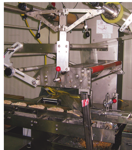
Above, the film-wrapped pizzas index into the cartoner, where pusher arms insert them into cartons the machine opens and prebreaks from blanks. Film overwrapper, right, runs the new film at lower temperatures with no rewrips.
