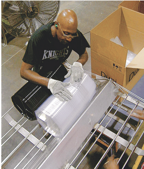
Roll-fed PS feeds two in-line thermoforming systems, above, that can handle molds up to 50×50 in., and up to a 7-in.-deep product. After thermoforming, the finished clamshells are counted by an operator at Duni, right.
