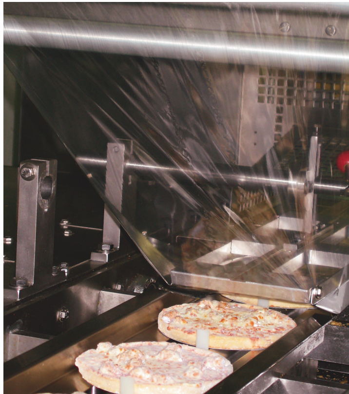
Frozen pizzas, below, single-file into a film-overwrapping system to be enclosed in clear PVC shrink film before conveying to a shrink tunnel.
